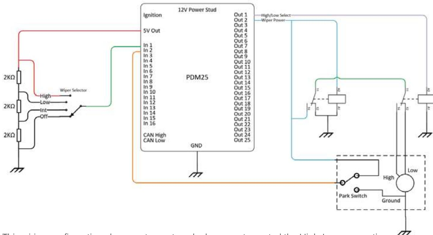
This wiring configuration also uses two external relays, one to control the High-Low connection to the motor and a second to control power to the motor.
