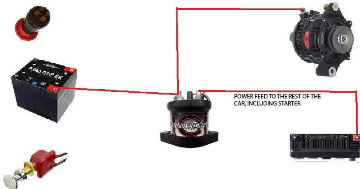
SINGLE CONTACTOR WITH ALTERNATOR POWER DISTRIBUTION DIAGRAM
